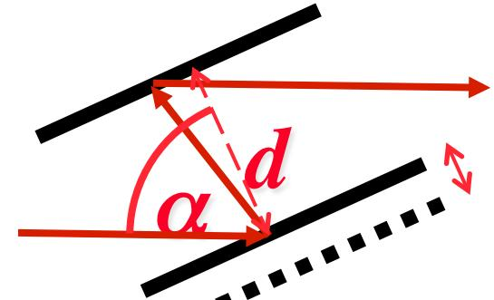
$$\left. \frac{\partial^2 \varphi}{\partial \omega^2} \right|_{\omega_0} = \text{GDD} = -d \frac{N^2 \lambda^3}{2\pi c^2} \cdot \frac{1}{\cos^3(\beta)}$$
