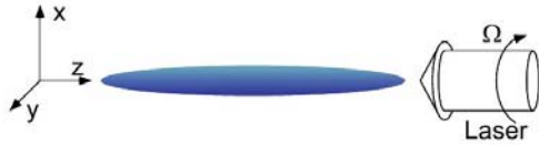
Figure 2: A cigar-shaped atomic cloud confined in an axisymmetric magnetic trap is stirred by a far-detuned laser beam. The laser beam propagates along the long axis of the cigar ( z ), and it creates a dipole potential which is anisotropic in the xy plane. This anisotropy rotates around the z axis at the angular frequency \Omega .
